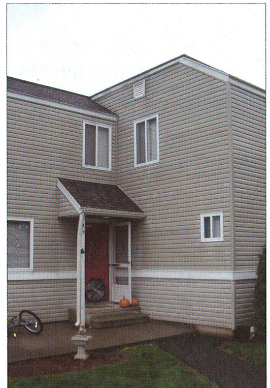
A blower door was set up in this typical townhouse unit. Testing indicated substantial leakage under the porch roof.
