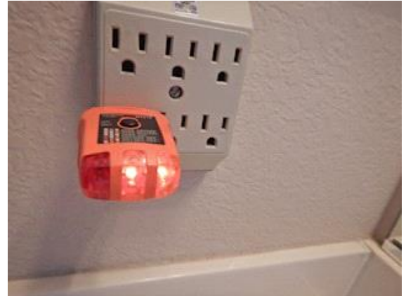
Bathroom 2: the outlet is GFCI protected, the GFCI is located in the garage
