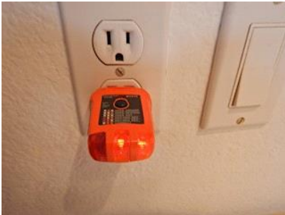
Bathroom 1: the outlet is GFCI protected, the GFCI is located in the garage
