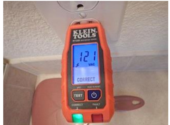
Bathroom 1: the outlet is GFCI protected
