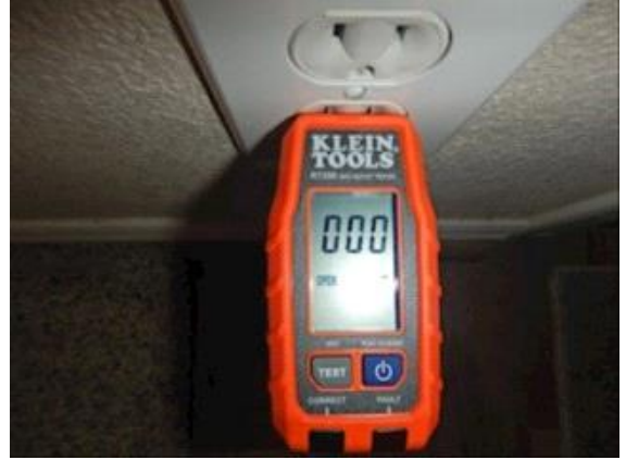
Living room: the outlet is showing an open hot
