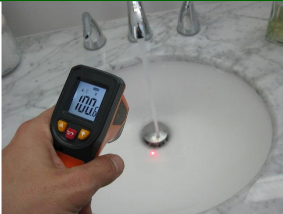
Water heater delivering hot water at time of inspection
