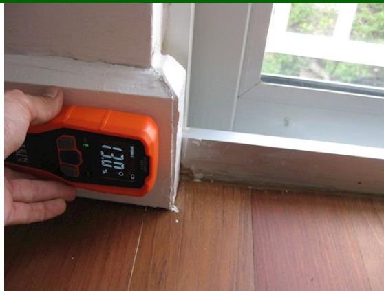
Humidity reading taken in main bedroom along baseboards near sliding glass door, areas was dry at time of inspection. Baseboards were seen separated from themselves most likely due to elevated humidity in the area as the sliding glass door does now have a weather strip
