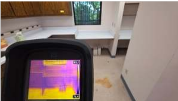
Current water detected at the laboratory wall
