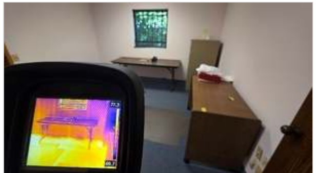
Current water detected at the south office wall
