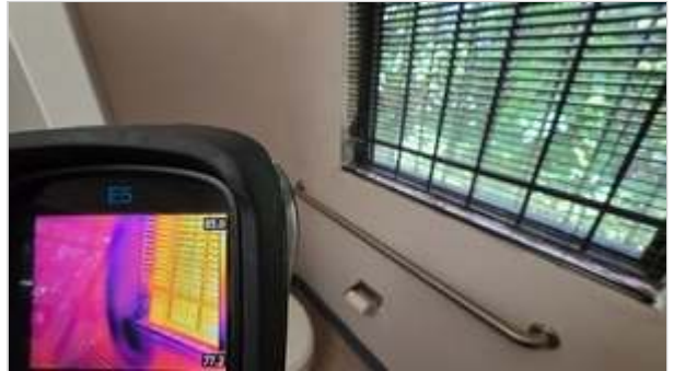
Current water detected at the south bathroom wall
