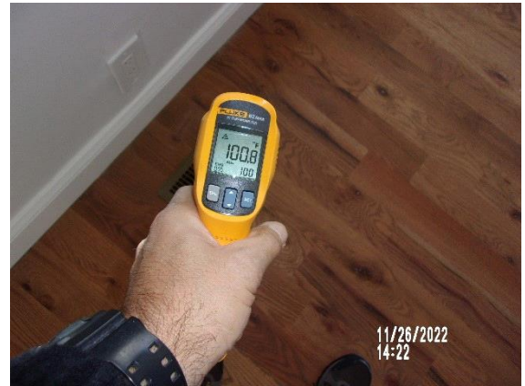
Heating Distribution: heat detected in all other registers on first floor.
