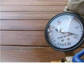
Water Pressure/Flow: Water flow was between 8 and 13 gallons per minute at three different hose bibs.
