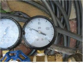
Water Pressure/Flow: Water pressure registered at about 40 psi at three different hose bibs.
