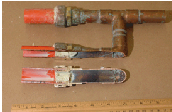
Cross Section of Dezincified Compression Fitting
