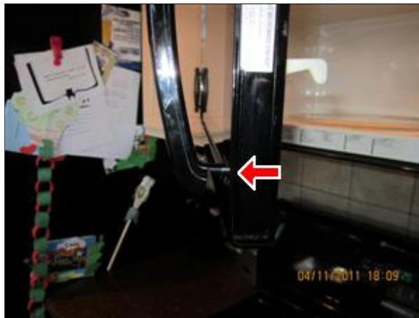
E. Picture 1 Handle broken on microwave
