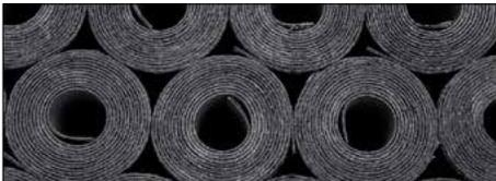
Until 35 years ago, asphalt products — including BURs — dominated the commercial roofing industry. In the early 1980s, the commercial roofing market began shifting to single-membrane roofing. Today, BUR is applied to about 20 to 25 percent of low-slope roofs on new commercial buildings, and a BUR system can be expected to last 20 to 30 years.
